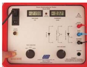
Place the function switch in the PRV (PFV) position and press the "TEST" button. Slowly increase the voltage while observing the Peak Voltage and Peak Leakage Current on the panel meters. In a properly functioning device, the rated voltage should be reached before the current starts to rise **rapidly**, (the "break-over point").
