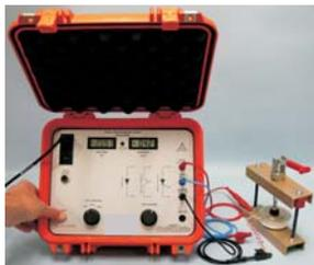
Set the Voltage Control to the zero position (fully counter clockwise) before turning the unit on. Connect the Anode, Gate and Cathode leads to the device to be tested.
