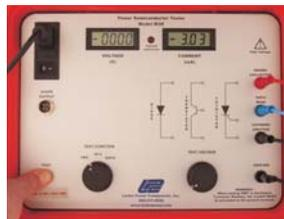
Place the function switch in the PRV position and press the "TEST" button. Slowly increase the voltage while observing the Peak Voltage and Peak Leakage Current on the panel meters. In most transistor modules, the current will rise immediately due to the circuit design.
