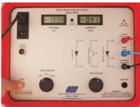
Place the function switch in the PRV position and press the "TEST" button. Slowly increase the voltage while observing the Peak Voltage and Peak Leakage Current on the panel meters. In a properly functioning device, the rated voltage should be reached before the current starts to rise **rapidly**, (the "break-over point").
