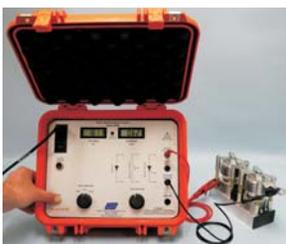
Make sure the Voltage Control is at the zero position (fully counter clockwise) before turning the unit on. Connect the Anode and Cathode leads to the diode to be tested.
