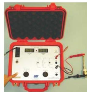
Make sure the Voltage Control is at the zero position (fully counter clockwise) before turning the unit on. Connect the Anode and Cathode leads to the diode to be tested.
