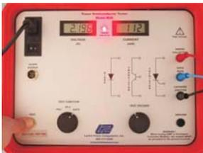
Place the function switch in the GATE position and slowly raise the Voltage Control while observing the "TRIGGER INDICATION" light. If the light does not turn on, the Gate on the SCR is faulty, and the device should be replaced.
