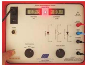
Place the function switch in the BASE position and slowly increase the voltage while observing the "TRIGGER INDICATION" light. If the light does not turn on, the Base is faulty, and the device should be replaced. Note: Typical turn-on voltage is 5-6 V. The current is so low in transistor base circuit, that it will not show on the current meter.
