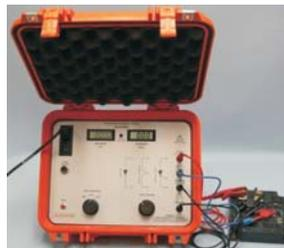
Connect a test lead between the ground plate of the component and the GROUND terminal on the tester.
