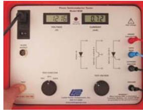
Place the function switch in the PFV position and press the "TEST" button. Slowly increase the voltage while observing the Peak Voltage and Peak Leakage Current on the panel meters. In a properly functioning device, the rated voltage should be reached before the current starts to rise rapidly, (the "break-over point").
